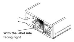
After inserting the disc, you can enter the original disc title to replace the disc number (see "Labeling discs (Disc Name)" on page 21) so you can locate it easily whenever you want to play it.
